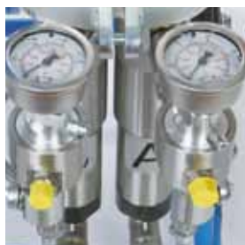
Pressure gauge units at machine outlet for component A and component B
