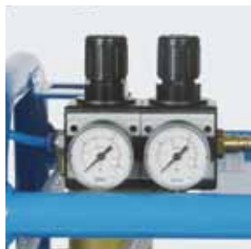
Manometers at pressure reducer for the components A + B and the rinsing pump
