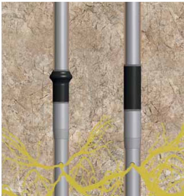
Tension of the rubber ring closes gap.
