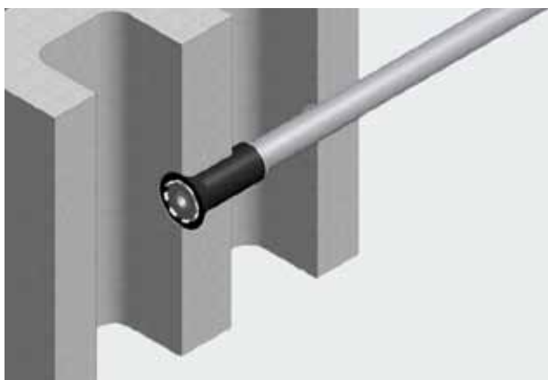
Injection packer clamped in the hollow brick
