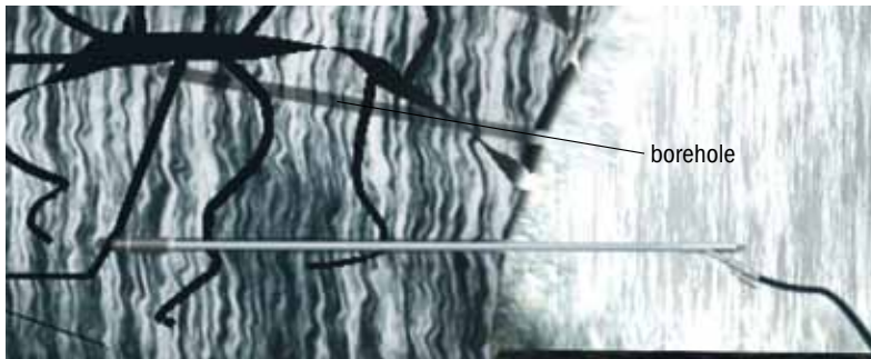
Place clamping packer and fix it using the clamping and injection device
