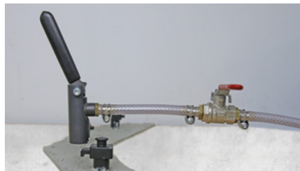
Slide the DESOI Z-Slider onto the pan head nipple
