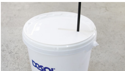
Position the dissolver mixer laterally within the slot
