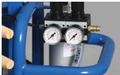
Manometer am Druckminderer Manometers at pressure reducer
